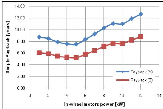
**Figure 8** Payback for different cars (wheel power = 5 kW, scenario A) (see online version for colours)
